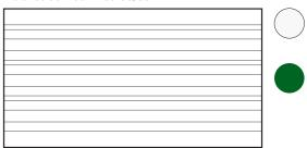
${\tt *Max.height\,of\,boards\,with\,these\,printed\,enamel}$ surfaces: 120 cm. The surface of enamelled steel boards smaller than 120 cm must be cut to size. The lines will therefore not be evenly spaced across the full height of the board.
